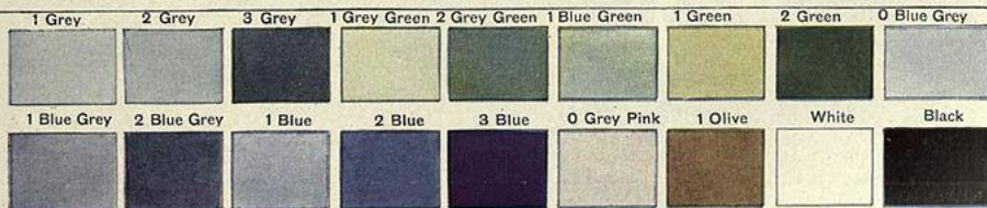
Colour chart issued to painting contractors showing the principal colours used in dazzle-painting.
